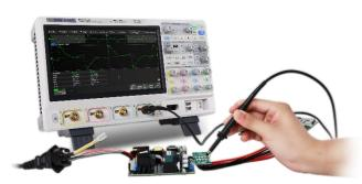
The SDS5000X can control the USB AWG module or a standalone SIGLENT SDG generator, to scan the amplitude and phase frequency response of the DUT, and display the data as a Bode Plot. This makes it possible to replace expensive network analyzer in some applications The Power Analysis option provides a full suite of power measurements and analysis, which greatly improve the measurement efficiency in switching power supplies and power devices design
