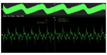
Using hardware-based Zoom technique and record length of up to 250 Mpts, users can select a slower timebase without compromising the sample rate, and then quickly zoom in to focus on the area of interest
