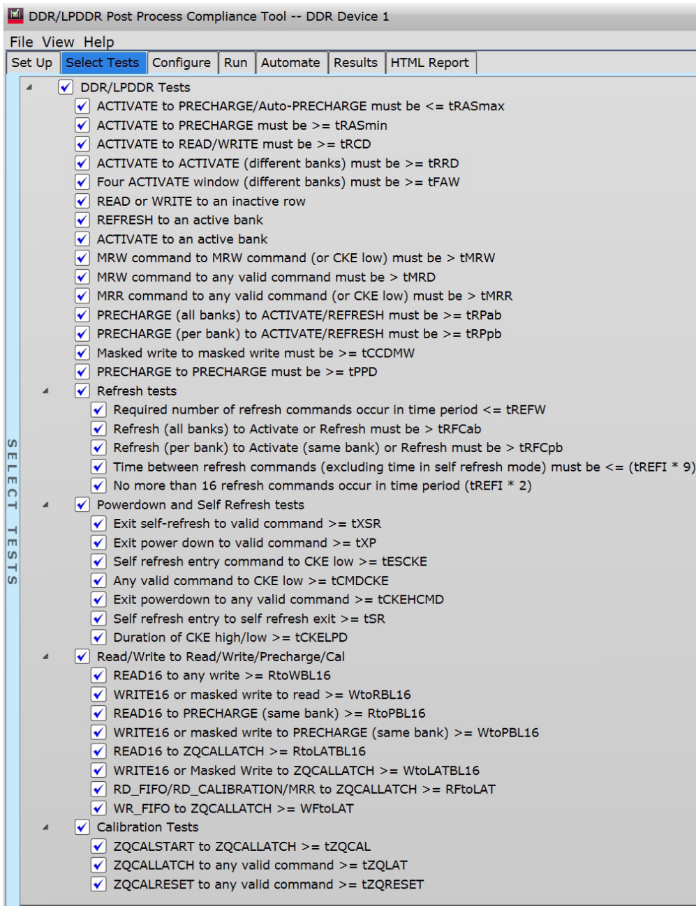
Figure 30. LPDDR4 post process compliance tests from B4661A Option -3FP/TP/NP.
