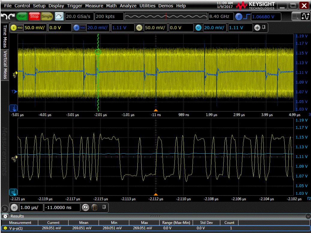
Figure 17. FPGA DC supply and the serial data captured by the S-Series oscilloscope. Data line (YELLOW trace); Power Supply (BLUE trace)
