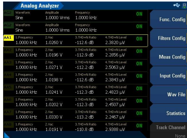
Figure 5. The U8903B's GUI, showing 8 analyzer channel measurements.
