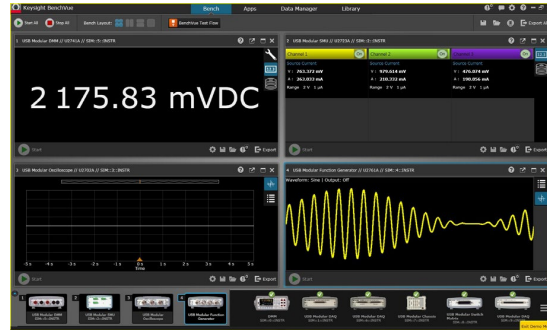
Figure 7. View measurements across USB DAQ, modular, and bench instruments all on one BenchVue interface.
