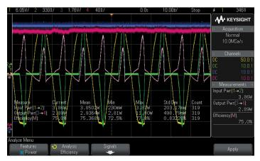
Figure 9. Efficiency analysis tests the overall efficiency of the power supply
