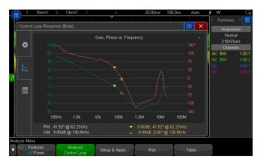
Figure 13. Control Loop Response gain measurement using an InfiniiVision X-Series oscilloscope.
