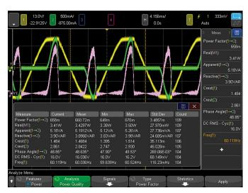
Figure 4. The power measurements option provides a results table with the following power quality measurements: Power Factor, Real Power, Apparent Power, Reactive Power, Crest Factor and Phase Angle.
