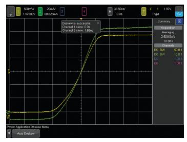
Figure 14. To make accurate power measurements and calculations, it is extremely important to null out the time delay between your voltage and current probes.
