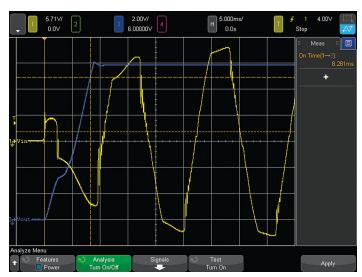
Figure 7. The turn-on analysis measures the time taken to get to the steady output voltage of the power supply after the input voltage is applied.
