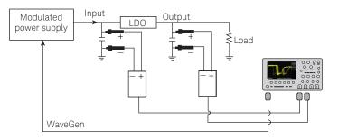
Figure 10. The PSRR is defined as the ratio of the output ripple compared to the input ripple over a wide frequency range.
