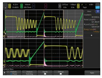
Figure 1. By measuring the switching loss and conduction loss, you can characterize the instantaneous power dissipation in a switching power supply.
