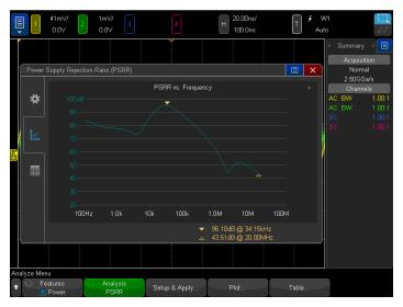
Figure 11. The PSRR is a measure of how well a circuit rejects ripple coming from the power supply input at various frequencies.
