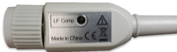
Figure 2. Low-frequency compensation adjustment (for N2840A/41A/42A/43A/53A)
