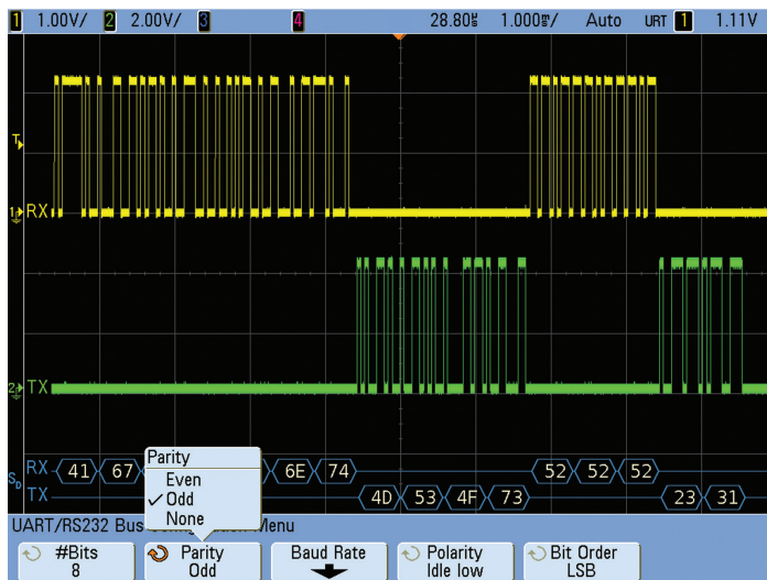
Figure 1. Defining the RS232/UART protocol structure
