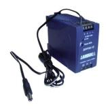
This power supply is supplied with a low voltage cable that plugs into the back of the Encore Series 61000 instrument. This power supply provides a 12 VDC output that powers the instrument and is capable of being secured to a DIN rail TS35/7.5 or TS35/15.
