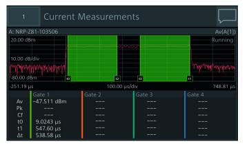
Determination of power of an EDGE burst using an R&S<sup>®</sup>NRPxxS(N) threepath diode power sensor and the gate function; exclusion of training sequence in the center of the signal
