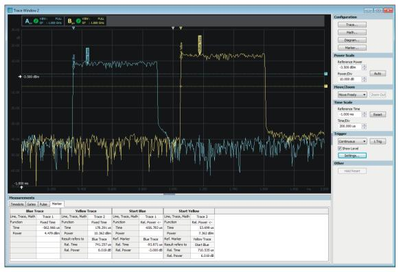
Pulse delay measurement on different traces
