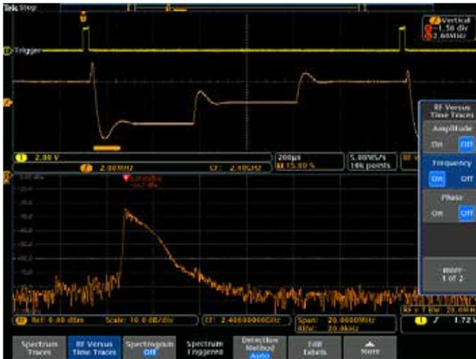
The orange waveform in the Time Domain view is the frequency vs. time trace derived from the spectrum analyzer input signal. Notice that Spectrum Time is positioned during a transition from the highest frequency to the lowest frequency, so the energy is spread across a number of frequencies. With the frequency vs. time trace, you can easily see the different frequency hops, simplifying characterization of how the device switches between frequencies.
