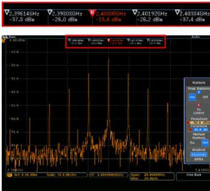
Automated peak markers identify critical information at a glance. As shown here, the five highest amplitude peaks that meet the threshold and excursion criteria are automatically marked along with the peak's frequency and amplitude.
