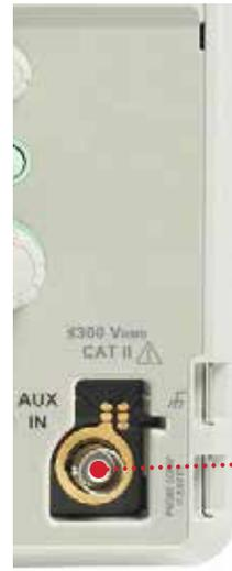
**AUX IN** on instruments without option SA3 or SA6 provides an auxiliary input for use as a trigger source
