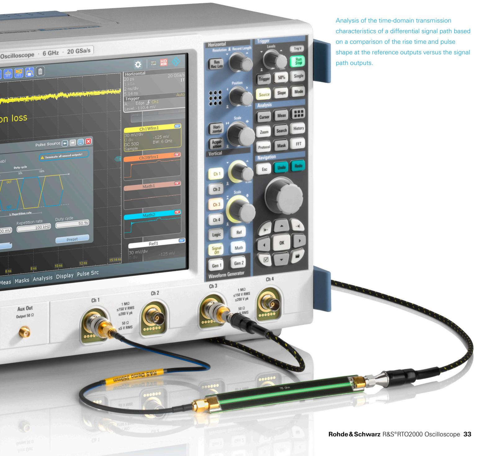
Analysis of the time-domain transmission characteristics of a differential signal path based on a comparison of the rise time and pulse shape at the reference outputs versus the signal path outputs.
