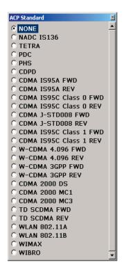
The R&S°FSL's wide scope of functions also extends to channel/adjacent channel power measurements. To simplify use, many default settings can be selected by pressing a button.
