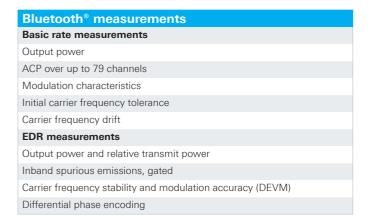
Adjacent channel power (ACP): This measurement determines the power of all adjacent channels. The power of up to 79 channels in total can be measured. For EDR inband spurious, the measurement can be gated.
