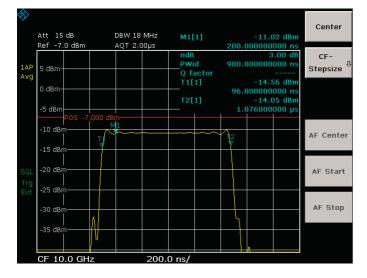
Typical applications of the R&S\*FSL18 include measurements in the microwave range, for example measuring the pulse width using the n-dB down marker.
