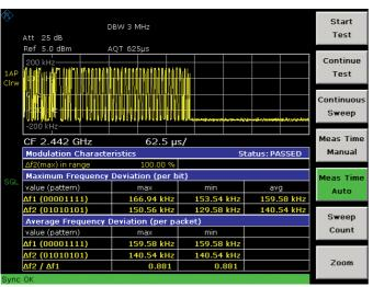
All measurements are carried out in line with the Bluetooth® RF Test Specification (Bluetooth® SIG) Rev. 2.0+EDR and cover basic rate as well as EDR. Integrated limit value monitoring is provided for all measurements and allows analysis of the results in the development and production of Bluetooth® modules.
