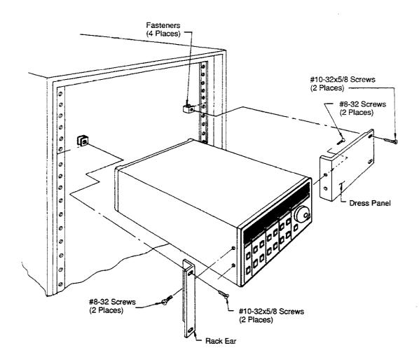
Figure 1. Single Rack Mounting Kit Installation
